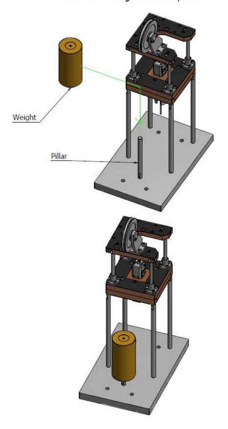
Attach the wire string to the upper plate and weight.
