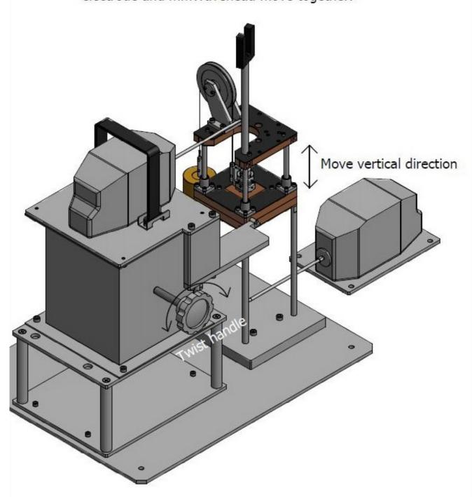
①Lift up BCDR upper electrode and remove the anti-rust paper.
