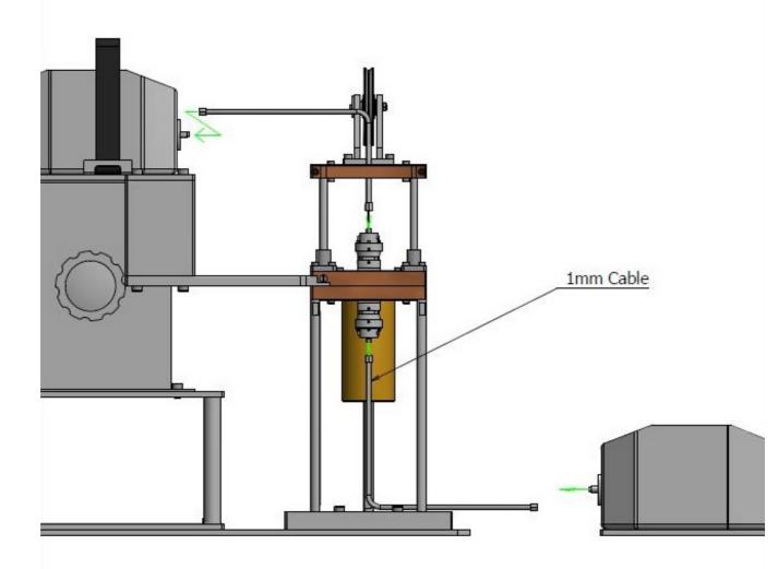
6 Twist the elevation handle to see the electrode and mmWavehead move together.
